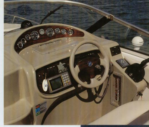
(above) The belm on the 268 is an exciting new look featuring full individual VDO instrumentation and generous room for custom electronics. Tilt-wheel, compass and walk-through windshield are standards.
