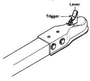
Figure S4: Coupling Assembly
