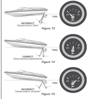
Figures T3-T5: Trimming the Boat with Outdrive
