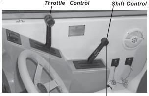
Trim Switches Detent Switch Figure F1: Gaffrig Shift and Throttle
