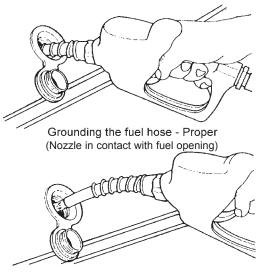
Not grounding the fuel hose - Improper (Nozzle not in contact with fuel opening)
