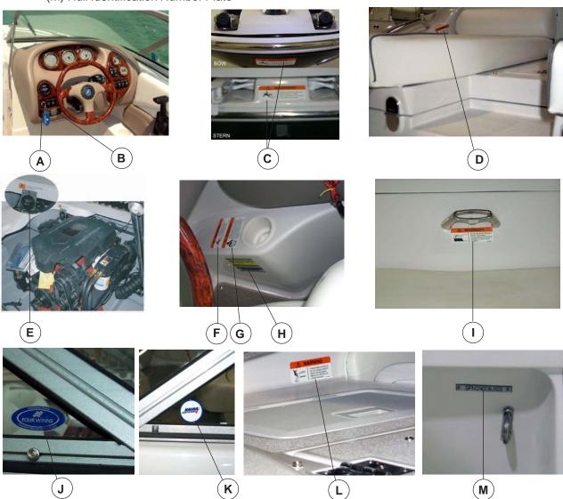
Figure 1: Freedom™/Horizon™ Models - Warning, Capacity and Other Label Locations (Reference Only)
