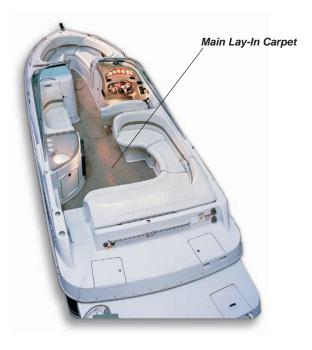
Figure N40: Cockpit Lay-in Carpet
