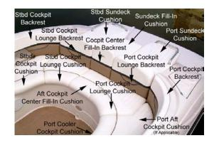
Figure N19: U-Wrap Aft Seating Note: Representative View - Seating may vary depending upon model.
