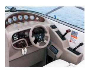
Figure E4: Helm Station - Twin Engine
