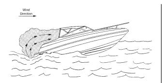
Figure B12: Operating at Slow Speed with Following Wind
