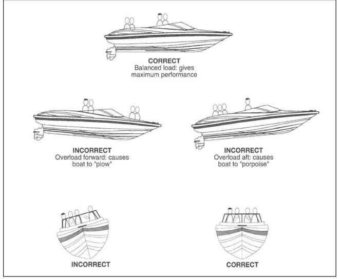
Figure T1: Loading Passengers and Gear
