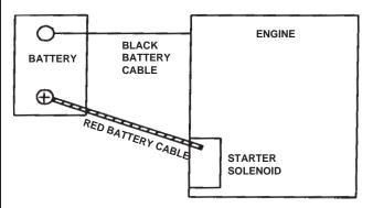
Figure H1: Single Engine-Single Battery Installation
