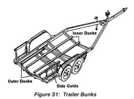
Outer bunk supports provide stability for the boat. The inside bunks are the main weight bearing members. Side guide-on supports help to keep the boat straight while driving the boat onto the trailer. Keeping the tie-downs tightly fastened will prevent the boat from bouncing against the bunk supports.
