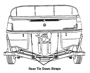
Figure S11: Rear Tie Down Straps
