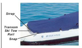
Figure O7: Cockpit Cover - Straps & Snaps
