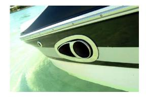
Figure M13: Thru-Hull Exhaust
