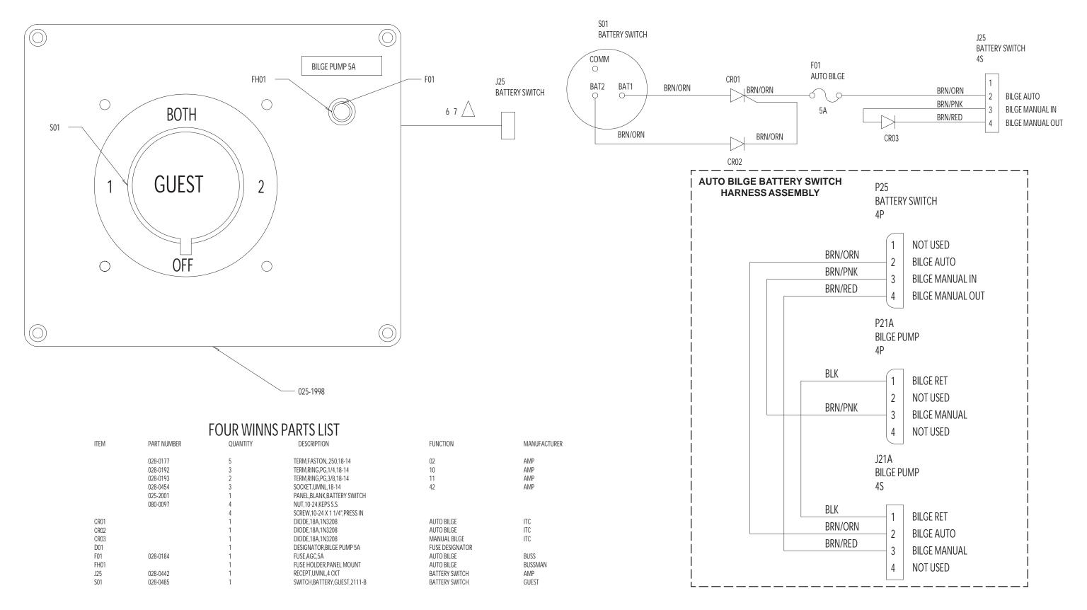
210/230/250 HORIZON OPTIONAL DUAL BATTERY W/ SWITCH PANEL ASSEMBLY Page 10
