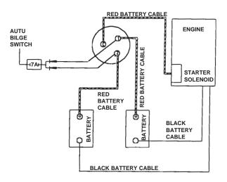
Figure H2: Single Engine-Dual Battery Installation
