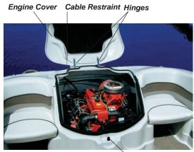
Figure N16: Engine Cover (Hinged Style)
