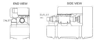
Figure J12: Vacu-flush™ Vacuum Generator
