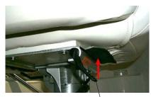
Lift adjustment lever up to move forward and back. Figure N6: Bucket Seat Slider
