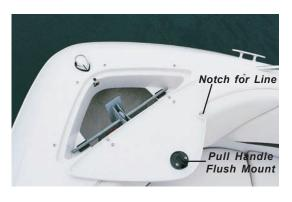
Figure L6: Anchor Locker
