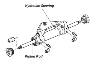
Figure G2: Hydraulic Steering
