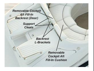
Figure N23: Walk-Thru Backrest Door & Fill-In Cushion
