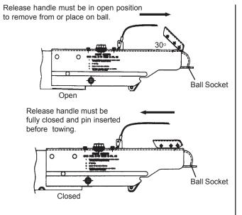
Figure S6: Surge Brake Actuator & Coupling Assembly
