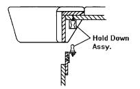
Figure N14: Hold-Down Assembly
